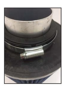
Wrap the 2mm thick rubber strip around the cone neck. There will be a 3 or 4mm gap which will close up when the hose clip is tightened (the hose clip will require loosening by turning the screw anti-clockwise, in order to fit over the strip AND the cone neck). Align the hose clip so that it overlaps the join in the strip.
