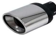
U 23 63 20 Tailpipe "SUPERIOR 63" Oval 90/140 mm, L= 255 mm
