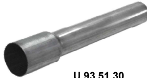
U 93 51 30 Decibel insert Should be placed inside piping in order to obtain an effective sound damping (note that this also leads to higher backpressure), L=283 mm
