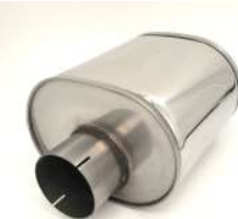
U 36 89 20R Silencer "OFFSETV 89" Oval 170/240 mm, L=250 mm (excl. ends)
