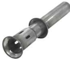
U 93 63 30 Decibel insert Should be placed inside piping in order to obtain an effective sound damping (note that this also leads to higher backpressure), L=275 mm
