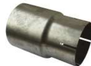
AA761603 Adaptor sleeve O/D 76.5 mm to I/D 60.3 mm L=120 mm
