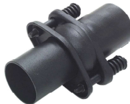
U 05 63 00 Compensator Should be used to prevent pipe fracture between the manifold and exhaust system, L=185 mm
