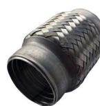
UFILOK60BMM Stainless steel flex-connector. Main body, stainless steel. End caps, aluminised steel L=101.6 mm/4". Fits over a 60.3mm pipe.
