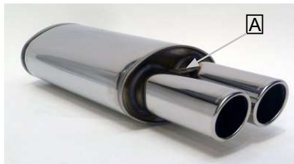
U 11 DJ DD Silencer "JETEX" Inlet pipe: 63.5 mm Oval silencer 140/220, L=420 mm Tailpipes Twin Round 80 mm, L=190 mm (excl. ends) Tailpipe width 165 mm Hanger point (A) 160 mm from end of tailpipes
