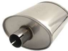
U 30 51 00R Silencer "TURBOTIGHT 51" Oval 140/220 mm L=250 mm (excl. ends)
