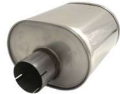
U 36 76 20R Silencer "OFFSET-V 76" Oval 170/240 mm, L=250 mm (excl. ends)
