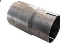
AA635511 Adaptor sleeve O/D 63.5 mm to I/D 50.8 mm L=105 mm
