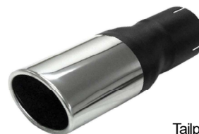
U 24 63 00 Tailpipe "QUATTRO 63" Square 70/90 mm, L= 270 mm
