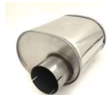
U 36 89 25R Silencer "OFFSETH+V 89" Oval 170/240 mm, L=250 mm (excl. ends)
