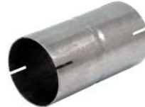
U 06 76 00R Double-end sleeve, L=150 mm I/D 3"
