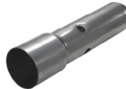
U 93 76 30 Decibel insert. Should be placed inside piping of at least 300 mm in order to obtain an effective sound damping (note that this also leads to higher backpressure), L=280 mm
