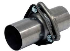
U 03 76 01R Three-bolt flange assembly Both ends 3" O/D, L=190 mm
