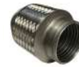
UFILOK38BMM Stainless steel flex-connector. Main body, stainless steel. End caps, stainless steel L=101.6 mm/4". Fits over a 1.75" pipe.
