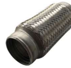
UFILOK57MM Stainless steel flex-connector. Main body, stainless steel. End caps, stainless steel L=152.4mm/6". Fits over a 57mm pipe.
