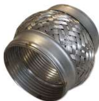
UFILOK89S Stainless steel flex-connector. Main body, stainless steel. End caps, aluminised steel L=101.6 mm/4". Fits over a 3.5" pipe.
