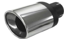
U 23 63 10 Tailpipe "ELLIPS XL 63" Oval 90/120 mm, L= 250 mm
